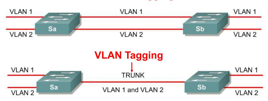
VLAN Tagging is used when a single link needs to carry traffic for more than one VLAN.
