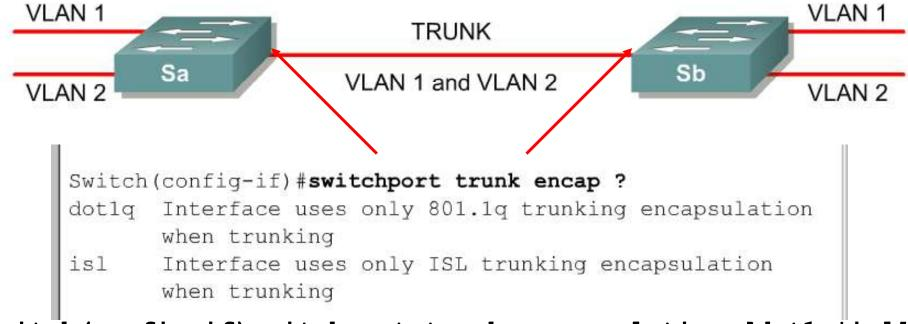
Switch (config-if) switchport trunk encapsulation [dot1q|isl]
