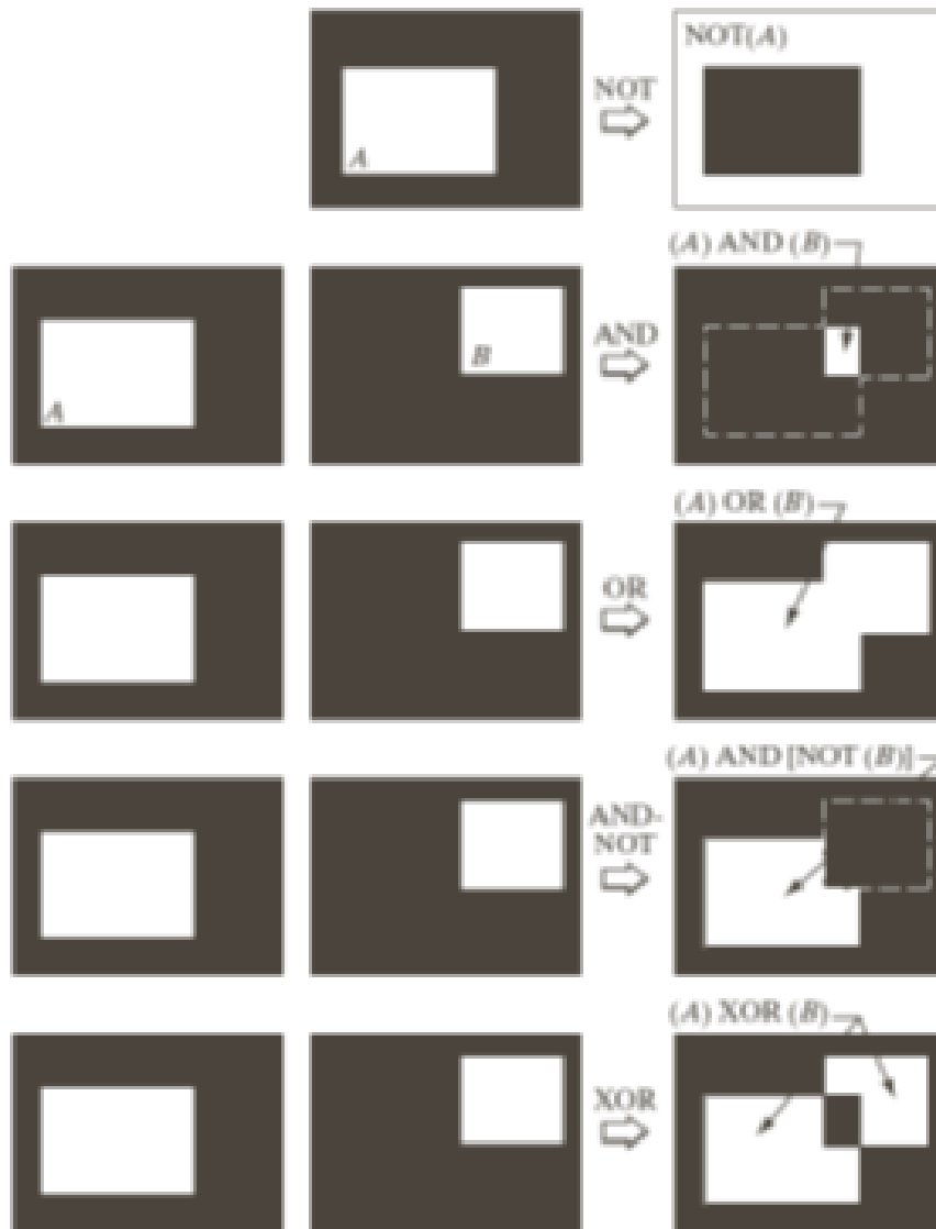
FIGURE 2.33 Illustration of logical operations involving foreground (white) pixels. Black represents binary 0s and white binary 1s. The dashed lines are shown for reference only. They are not part of the result.
