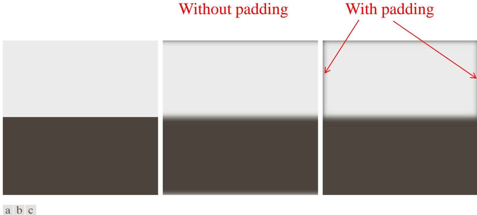
FIGURE 4.32 (a) A simple image. (b) Result of blurring with a Gaussian lowpass filter without padding. (c) Result of lowpass filtering with padding. Compare the light area of the vertical edges in (b) and (c).
