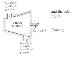
Analysis We take the turbine as the system. This is a control volume since mass crosses the system boundary during the process. We observe that there is only one inlet and one exit and thus  $\dot{m}_1 = \dot{m}_2 = \dot{m}$ . Also, work is done by the system. The inlet and exit velocities and elevations are given, and thus the kinetic and potential energies are to be considered.
