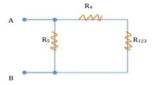
R<sub>123</sub> and R<sub>4</sub> are conncted in Series, Thus R<sub>1234</sub> is  $R_{1234} = R_{123} + R_4 = 5 + 20 = 25\Omega$
