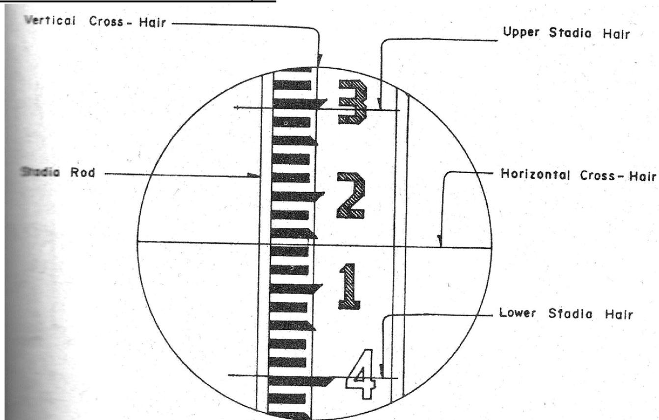
Fig. 2-1. Determining stadia interval on level rod.
