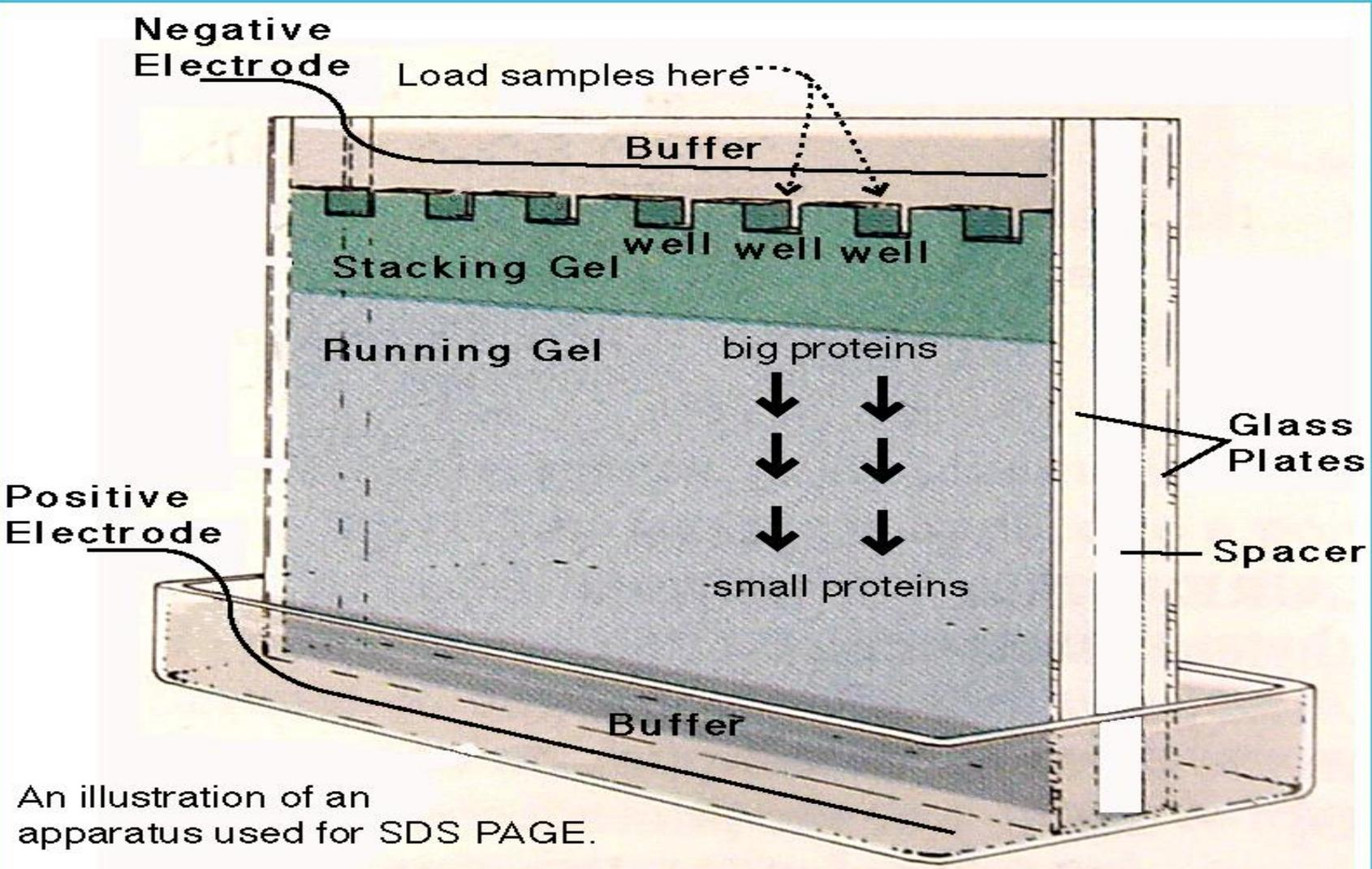
An illustration of an apparatus used for SDS PAGE.
