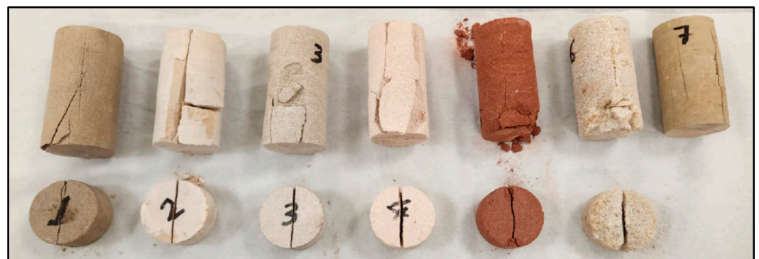
Figure 9. Core samples from various formations: after testing.
