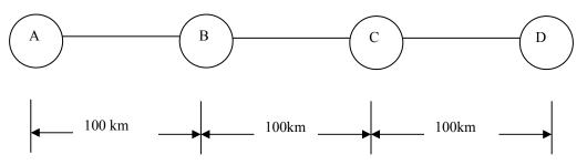
A is the sender and D is the receiver. Packets (if packet switching) traverse from A through B to C. Assume that headers for packet switching are 1000 bits. Assume the propagation rate is  $d = 10^3$  km/sec for both path AB and path BC. Channel speed for each path is:
