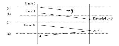
Assume that at time (a), the sender's window is empty and that the receiver's window contains 0, 1. A sends frames one by one. Frame 0 is lost on the way; frame 1 is
