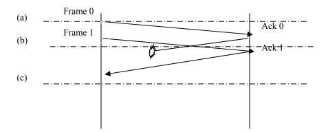
Assume that at time (a), the sender's window is empty and that the receiver's window contains 0, 1. A sends frames one by one. All frames (frames 0,1) are received by B without any loss/error. Acknowledgement for frame 0 is lost; A receives Acknowledgement for frame 1 successfully.
