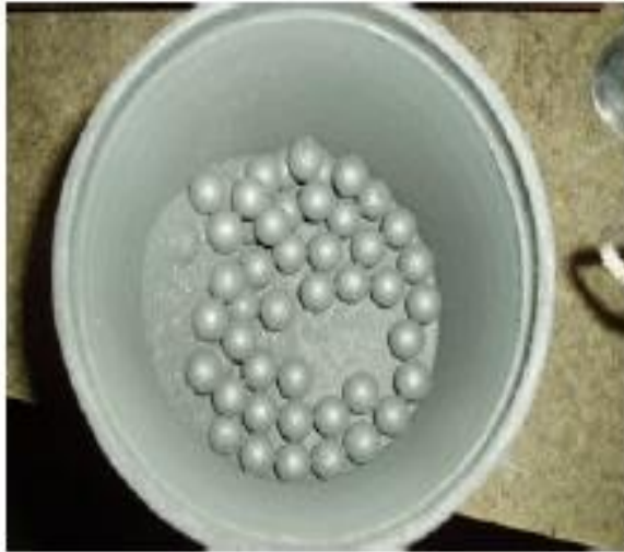
Lead antimony grinding media with aluminum powder
