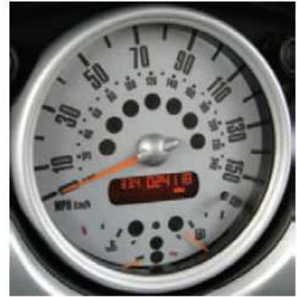
Figure 1.3 The speedometer of a vehicle that shows speeds in both miles per hour and kilometers per hour.
