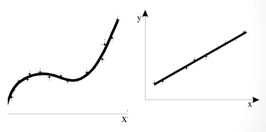
Wheb we draw a curve we cannot extend beyond the leftmost or rightmost points even if we know the mathematical form of the curve because we do not know if this is true for the device we operate.
