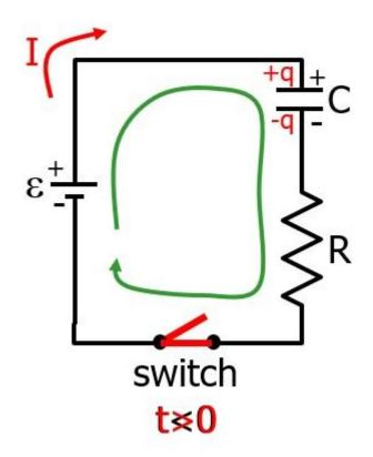
\*Convention for capacitors is "like" batteries: negative if going across from + to -.
