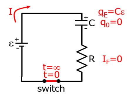
\*q=0 at t=0 only if the capacitor is initially uncharged (read the problems carefully!)
