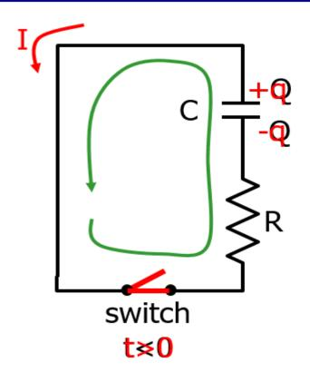
\*Convention for capacitors is "like" batteries: positive if going across from - to +.
