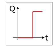
The approximation resulting from this assumption is reasonable, provided the resistance between the emf and the capacitor being charged/discharged is small.
