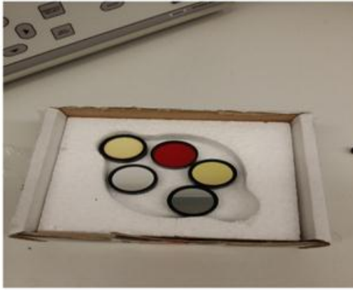
Figure 3: Five filters used to analyse the power conversion efficiency of solar cells in ultraviolet, visible, and near infrared region of the solar spectrum.
