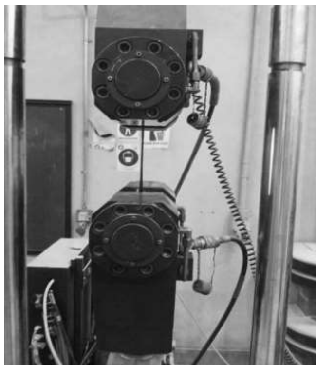
Figure 1. The setup of tensile test
