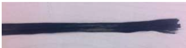
Figure 2. Carbon textile reinforcement uni-direction 50k.
