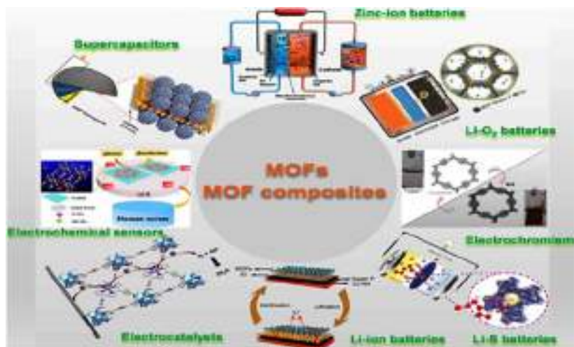
FIGURE 14.1 Schematic diagram of MOFs and MOF composites for electrochemical applications [31]. MOF , Metal-organic framework.
