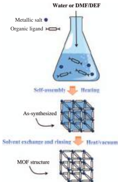
FIGURE 12.3 Schematic illustration of the solvothermal process.
