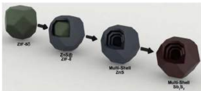
FIGURE 8.1 Schematic illustration route of synthesis to obtain multishell \text{Sb}_2\text{S}_3 from ZIF-8. Reprint with the permission from Xie F, Zhang L, Gu Q, Chao D, Jaroniec M, Qiao SZ. Multishell hollow structured \text{Sb}_2\text{S}_3 for sodium-ion batteries with enhanced energy density. Nano Energy 2019;60:591–9. ©2019, Elsevier.
