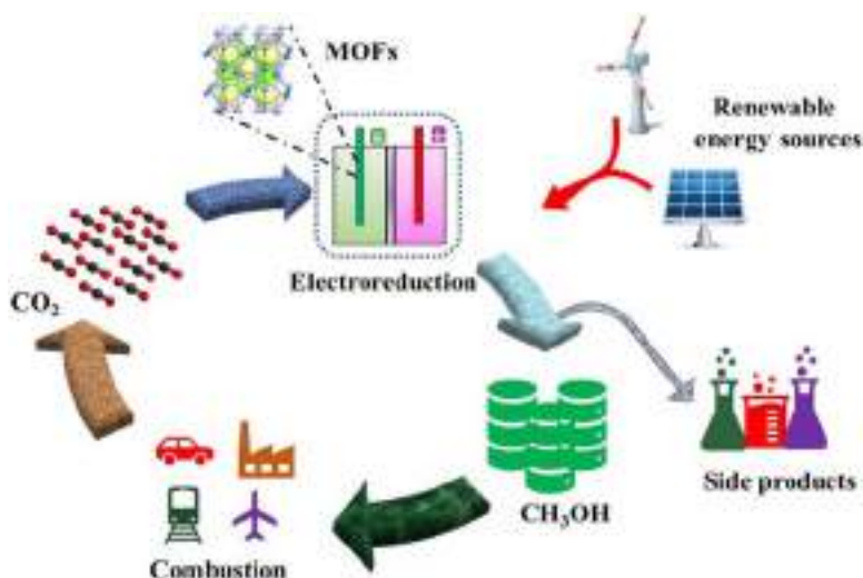
FIGURE 13.6 Pictorial representation of electrochemical reduction of CO 2 and probable of fuel product or chemicals [60].
