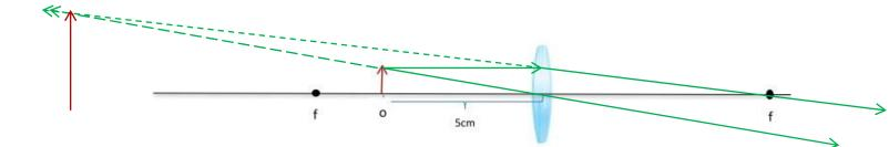
b)  $1/f = 1/d_0 + 1/d_i$  $1/7 = 1/5 + 1/d_i$ ,  $1/d_i = 1/7 - 1/5 = -2/35$ ,  $d_i = -17.5$  cm then the image created in front of the lens
