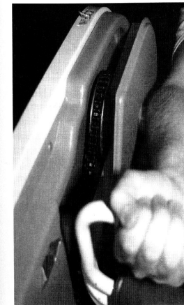
The Nautilus machine for the forearm flexors is shown in (A) above. A photograph of the actual cam is also presented. This machine uses a cam system which changes the moment arm of the weight, making it easier (B) or harder (C) to lift.
