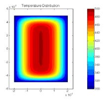
Temperature across a 2D plate in a time-stepping simulation with a Dirichlet boundary condition.
