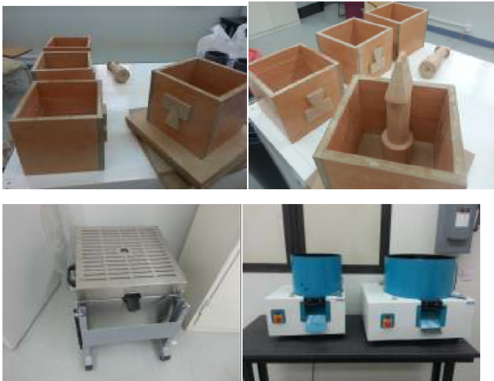
Fig. 2.8 Given green sand molding tools and equipment at the Industrial Engineering Department, “flakes, electric furnace, pattern and core box, and sand mixer/miller,.
