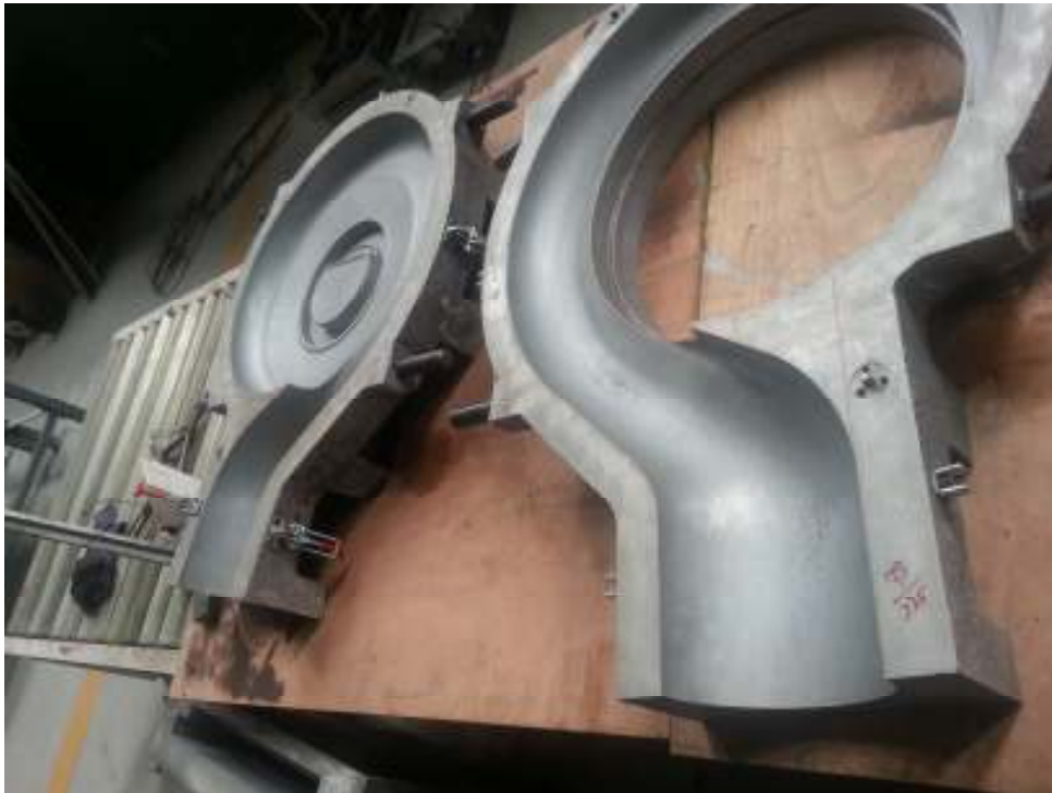
Fig 2.6 Cold split core box for big pump casing.
