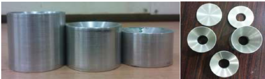
Fig. 1.10 Side and top view of die for rod extrusion process
