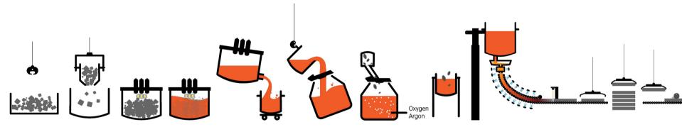
The **raw material** – recycled stainless steel and ferro-alloys – is transformed into **molten metal** in an electric arc furnace with a **melting capacity up to 160 tonnes.**
