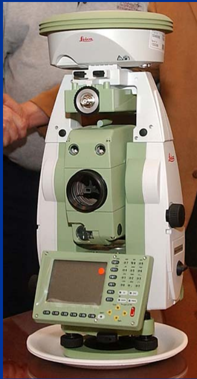
Total station equipped With Static GPS receiver
