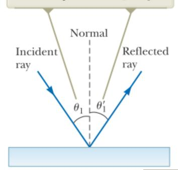
(The normal is a line drawn perpendicular to the surface at the point where the incident ray strikes the surface.)
