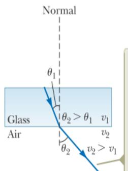
When the beam moves from glass into air, the light speeds up upon entering the air and its path is bent away from the normal. The ray that enters the second medium changes its direction of propagation at the boundary and is said to be refracted.
