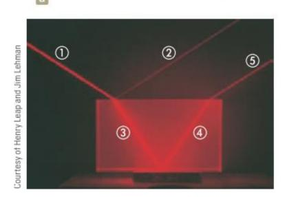
When the light beam moves from air into glass, the light slows down upon entering the glass and its path is bent toward the normal.
