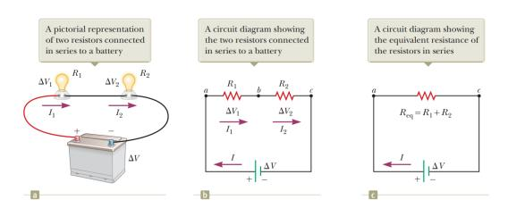
When two or more resistors are connected together as are the light-bulbs in the figure, they are said to be in *series*.
