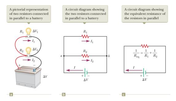
In this figure, When the current I reaches point a, called a junction, it splits into two parts, with  $I_1$  going through  $R_1$  and  $I_2$  going through  $R_2$ . A junction is any point in a circuit where a current can split,
