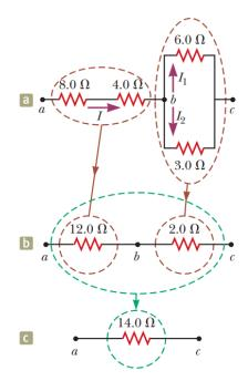
**Example-2:** Three resistors are connected as shown in the Figure. A potential difference of 18.0 V is maintained between points a and b.
