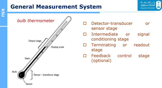
□These stages form the bridge between the input to the measurement system and the system output.
