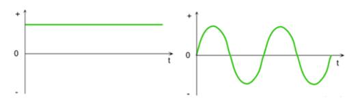
An ac circuit consists of circuit elements and a power source that provides an alternating voltage  $\Delta v$ . This time-varying voltage from the source is described by
