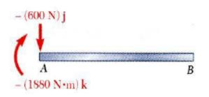
b) Find an equivalent force-couple system at B based on the force-couple system at A.
