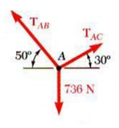
Free-Body Diagram: A sketch showing only the forces on the selected particle.
