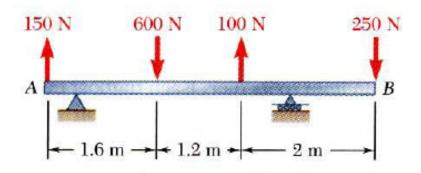
For the beam, reduce the system of forces shown to
