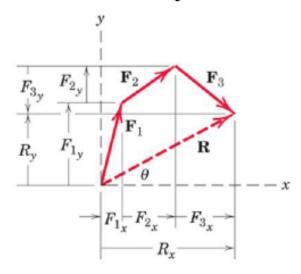
Magnitude and direction of the resultant force R is obtained by forming the force polygon where the forces are added head to
