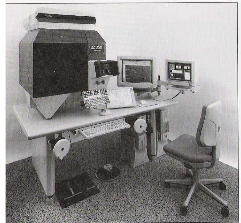
FIGURE 12-18 Leica SD3000 analytical plotter. (Courtesy LH Systems, LLC.)
