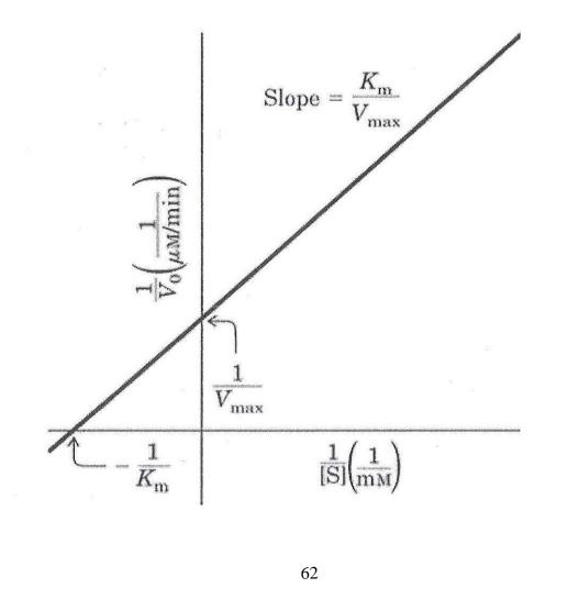
Both Vmax and Km can be obtained accurately from the intercepts of the straight line with the y-axis and x-axis.
