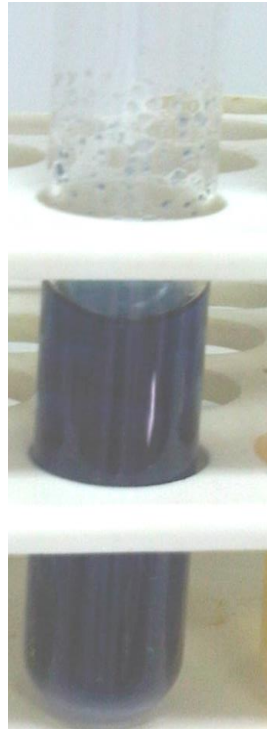
Starch + iodine [before heating]
