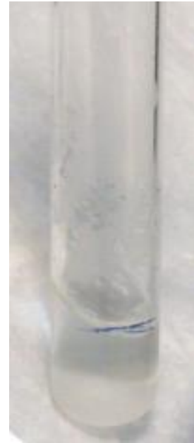
Starch + iodine [after heating]
