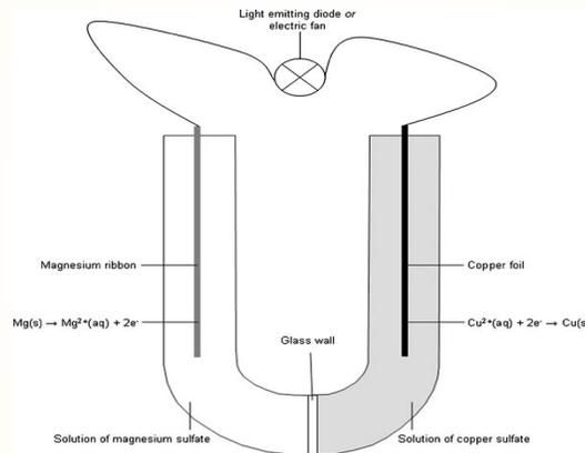
*Figure 1. The electrochemical cell setup in the practical.* Particulars of this cell include, among other things, the actual species of electrodes and solutions. Contingencies that occurred in the cell include, among other things, (a) success or failure in observing a copper precipitation on the copper foil, (b) a precipitation in and discoloration of the magnesium sulfate solution, (c) the fan and the LED either working or not, and (d) bubbles of hydrogen gas
