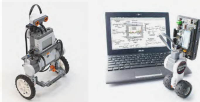
Self-balancing robots using LEGO and Arduino
