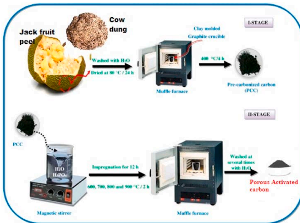
Scheme 1. Two stage preparation strategy of phosphoric acid activated PCC from Cow dung and Jackfruit peel waste (AP).
