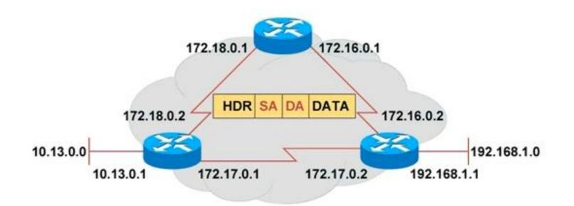
Unique addressing allows communication between end stations.
