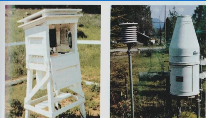
Figure 3.2 (a) A thermometer shelter. This white wooden louvered box houses maximum-minimum thermometers and other instruments. (b) A maximum-minimum temperature instrument system appears on the left side of this photo. To the right is a large recording rain gauge.
