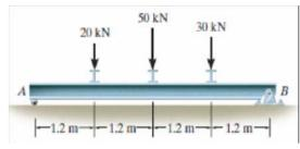
The timber beam has a rectangular cross section. If the width of the beam is 150 mm, determine its height h so that it simultaneously reaches its allowable bending stress of  $\sigma_{\rm allow} = 10$  MPa and an allowable shear stress of  $\tau_{\rm allow} = 0.35$  MPa. Also, what is the maximum load P that the beam can then support?
