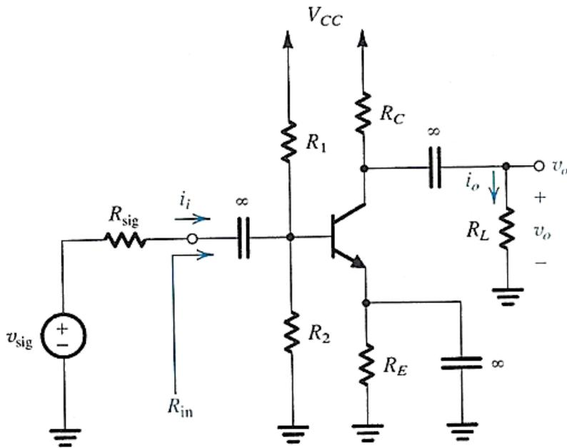
We first draw the DC equivalent circuit (all caps are open-circuited), then we find Thevenin's equivalent looking out of the base.
