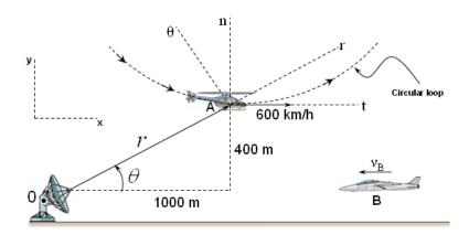
At the bottom of a circular loop in the vertical plane, at an altitude of 400 m, the helicopter **A** has a constant velocity of 600 km/h. The radius of curvature of the circular loop is 1200 m. For the radar tracking at **O**, determine
