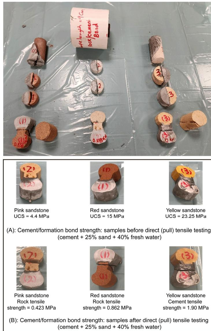
**Figure 8.** Test samples used to measure cement–rock sheath bond strength.
