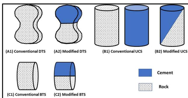
Figure 5. Adaption of conventional rock mechanical tests.
