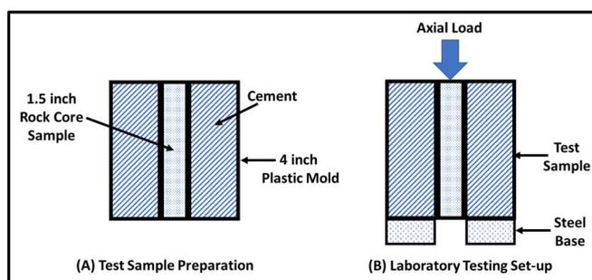
Figure 4. Cement–formation bond strength testing set-up.
