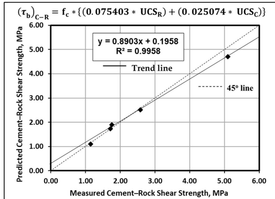
Figure 11. Measured and predicted cement–rock shear bond strength.
