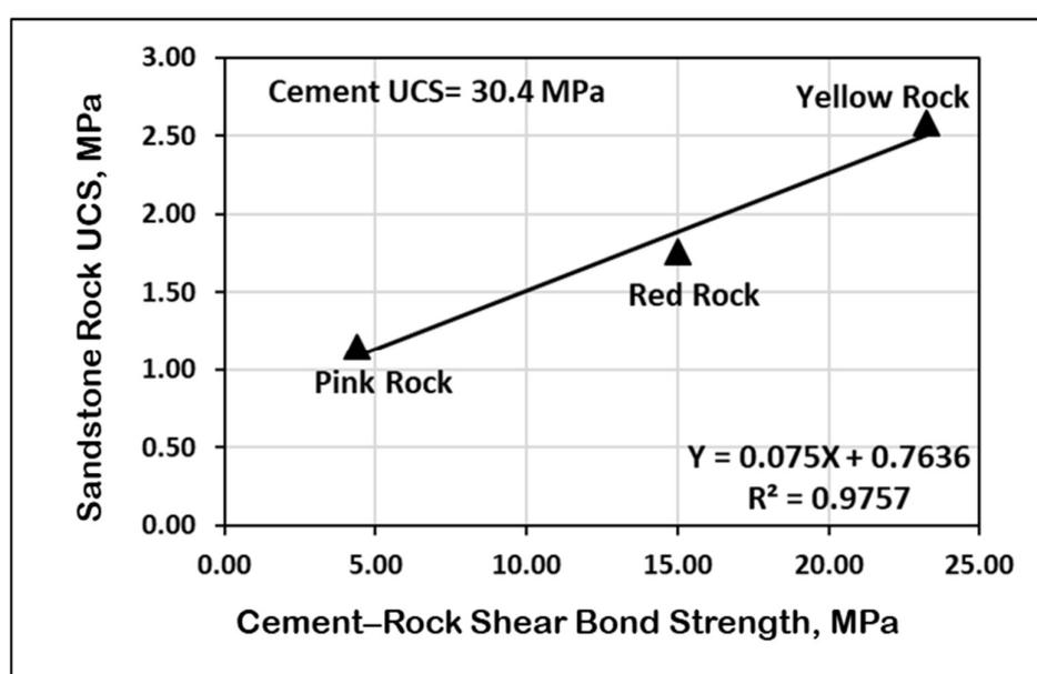
**Figure 9.** Relationship between rock UCS and cement–rock sheath bond strength.
