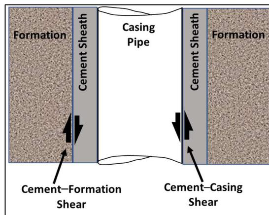
**Figure 1.** Cemented casing configuration.
