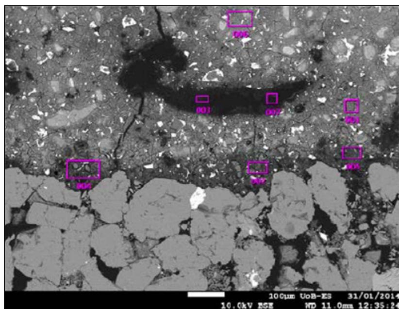
**Figure 10.** SEM image showing the presence of mud at the cement–rock interface (top: cement, bottom: rock) [26].
