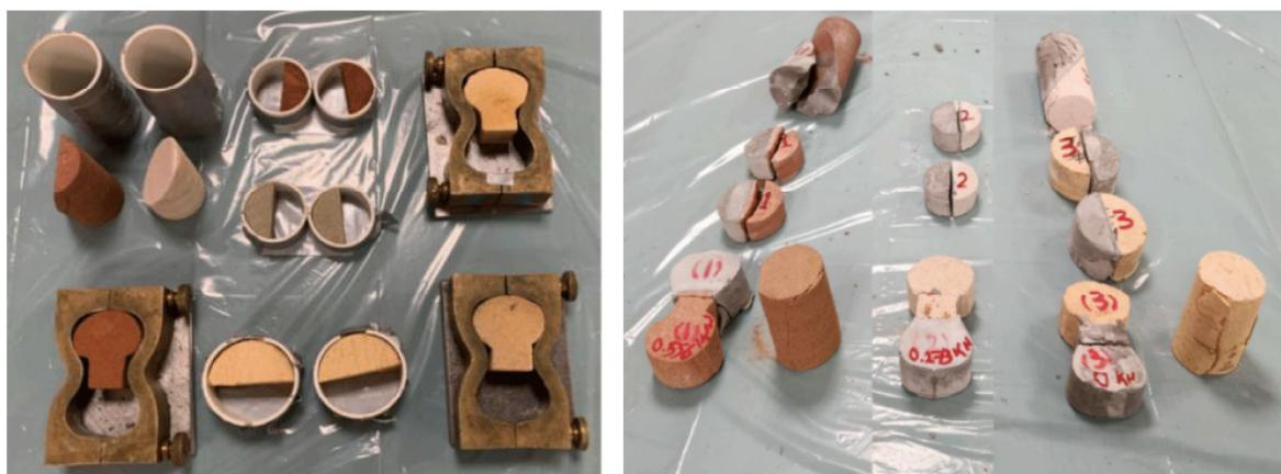
Figure 7. Unconventional method for cement–rock sheath bond strength measurement.
