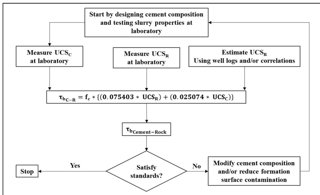
Figure 12. Cement–formation shear bond strength prediction process.
