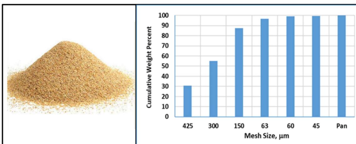
**Figure 3.** Granulometric analysis of the utilized local Saudi sand.
