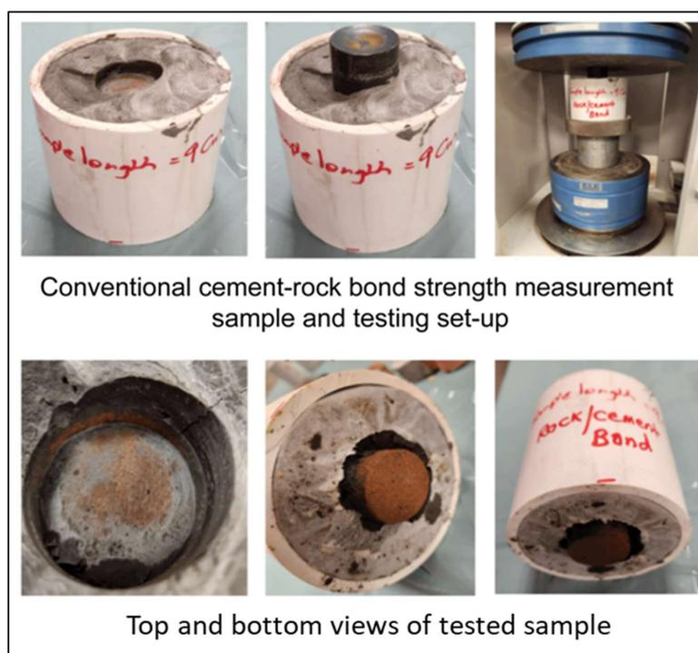
**Figure 6.** Simulated cement–rock sheath bond strength measurement.
