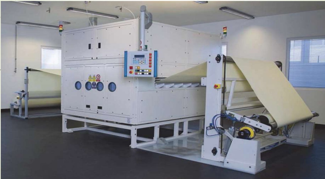
Nozzle-less production electrospinning line (Nanospider TM )
