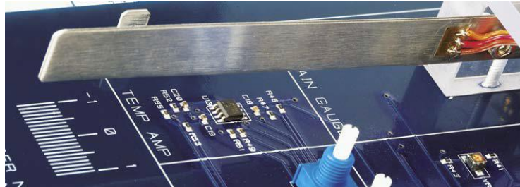
Figure 3.1: Strain gage measuring deflection of flexible link on QNET mechatronic sensors trainer
