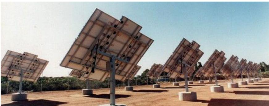
**Fig. 8** SAST concentrator solar cell array [26]
