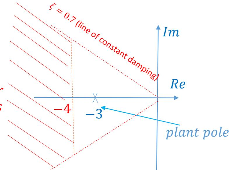
$$CLTF = \frac{\left(K_P + \frac{K_I}{s}\right) \left(\frac{10}{s+3}\right)}{1 + \left(K_P + \frac{K_I}{s}\right) \left(\frac{10}{s+3}\right)} = \frac{10(K_P s + K_I)}{s^2 + 3s + 10(K_P s + K_I)} \Rightarrow CLCE = s^2 + (10K_P + 3)s + 10K_I = 0$$
