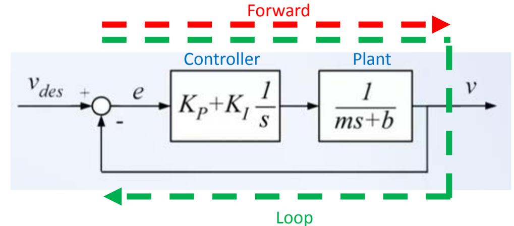
$$\frac{V(s)}{V_{des}(s)} = \frac{\text{forward}}{1 + \text{loop}} = \frac{(K_p + K_I \frac{1}{s})(\frac{1}{ms + b})}{1 + (K_p + K_I \frac{1}{s})(\frac{1}{ms + b})} = \frac{K_p s + K_I}{s(ms + b) + K_p s + K_I} = \frac{K_p s + K_I}{m s^2 + (b + K_p)s + K_I}$$
