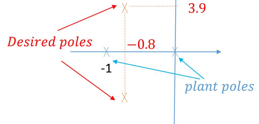
$$CLTF = \frac{(K_P + sK_D)\left(\frac{1}{s^2 + s}\right)}{1 + (K_P + sK_D)\left(\frac{1}{s^2 + s}\right)} = \frac{(K_P + sK_D)}{s^2 + s + (K_P + sK_D)} \Rightarrow CLCE = s^2 + s + (K_P + sK_D) = 0$$
