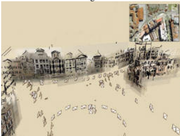
Figure 28 Screenshots from the explorer interface, showing location and orientation of various cameras. (Sanavely, et al 2006)
