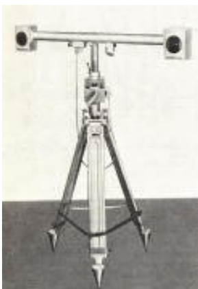
Figure 3 Zeiss SMK 120 set in normal position with the base and the lines of sight in the horizontal plane. (UNESCO, 1972)
