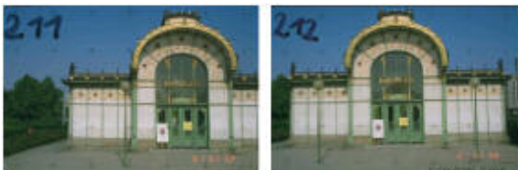
Figure 4 stereo pair images; 3D geometry can be reconstructed as long as the area of interest is seen in both images (from CIPA Otto Wagner Pavilion Karlsplatz, Vienna). (Grussenmeyer, et al., 2002)
