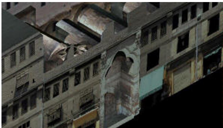
Figure 37 3D reconstruction isometric view of the building; textures derived from the photos are applied to the generated 3d model and referenced with the total station to produce a full textured 3D reconstruction. (ECAE, 2005)
