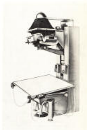
Figure 6 Optical rectifications; Optical rectification is done using photographic enlargers, developed by Carl Zeiss. (UNESCO, 1972)
