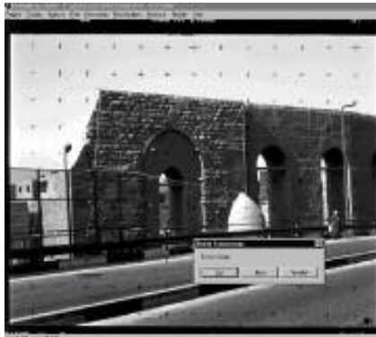
Figure 12 Digital rectification; MSR software is the most famous professional software in digital rectification. (Grussenmeyer, et al, 2002)
