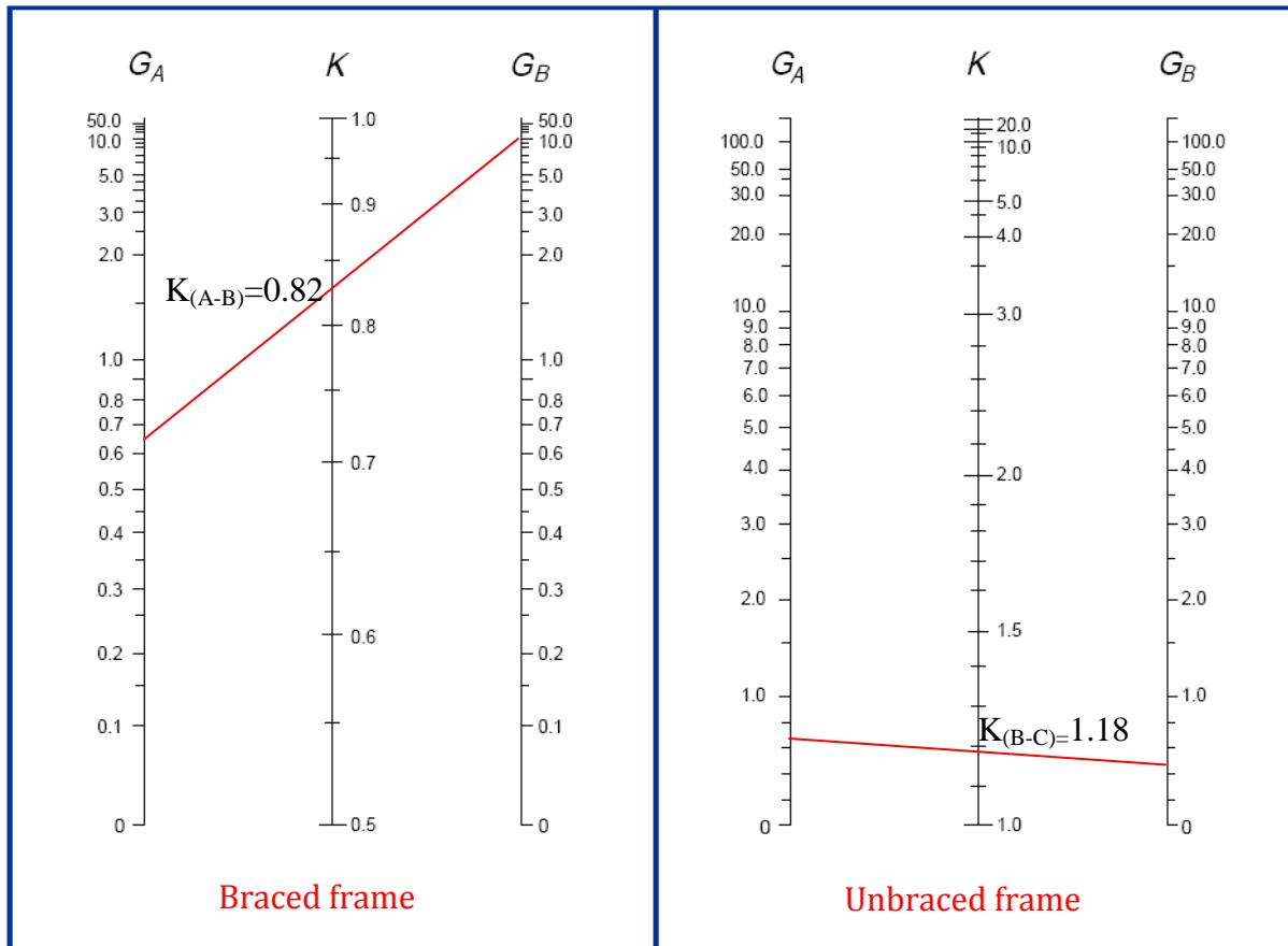
The subscripts \$A\$ and \$B\$ refer to the joints at the two ends of the column section being considered. \$G\$ is defined as
