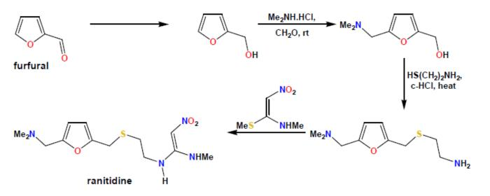
• Furfural is produced very cheaply from waste vegetable matter and can be reduced to give the commercially available compound furfuryl alcohol.
