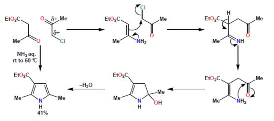
• A modified version of the Feist-Benary synthesis and using the same starting materials: an a-halo carbonyl compound and  $a_{\beta}$ -keto ester.
