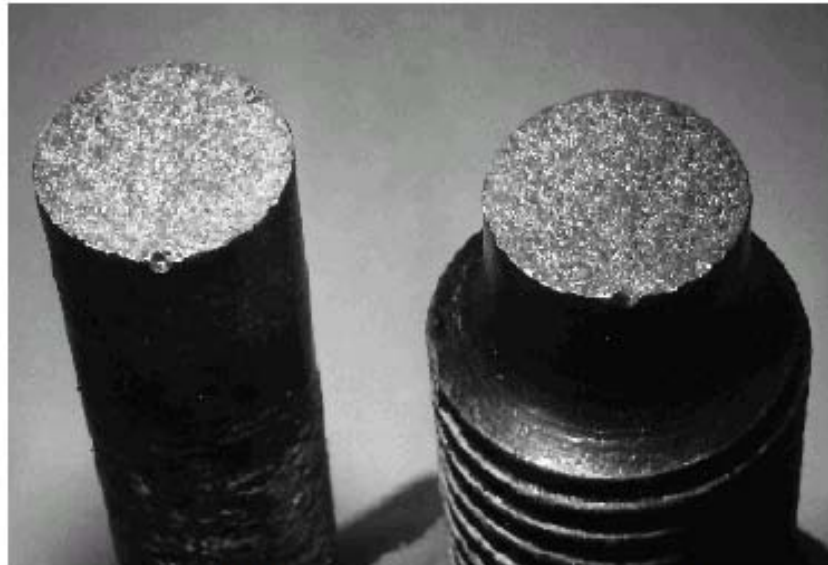
Brittle fracture in a mild steel
