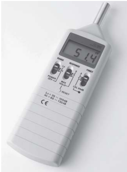
Typical handheld sound level meter (typically supplied with built-in frequency filter, the A filter )
