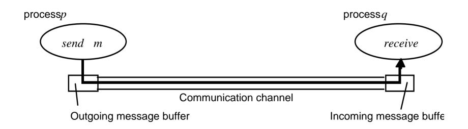
Communication channel proceduces an omission failure if it does not transport a message from "p"s outgoing message buffer to "q"'s incoming message buffer. This is known as "dropping messages" and is generally caused by lack of buffer space at the receiver or at gateway or by a network transmission error.
