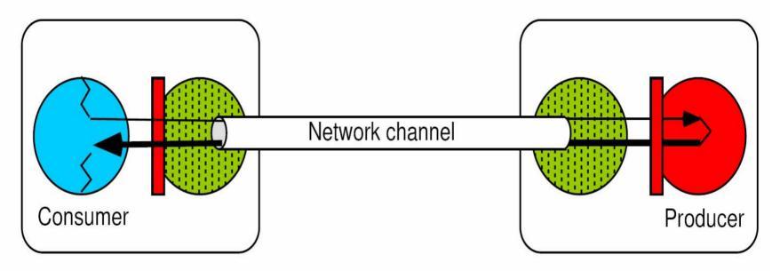
Node 1 The consumer performs a synchronous call, which is processed asynchronously by the producer.
