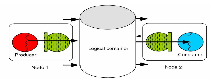
producers insert data asynchronously into the shared space, while consumers read data synchronously.
