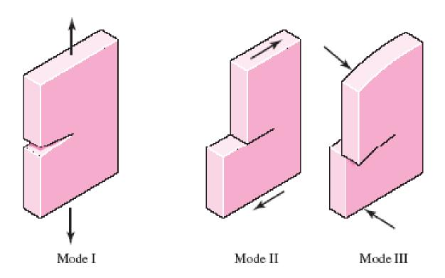
Consider a mode I crack of length 2a in the infinite plate of Fig. 5–24. By using complex stress functions, it has been shown that the stress field on a dx dy element in the vicinity of the crack tip is given by
