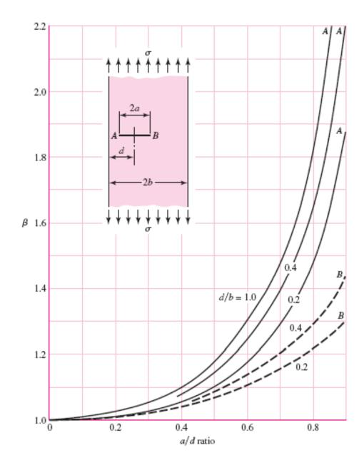
Plate loaded in longitudinal tension with a crack at the edge; for the solid curve there are no constraints to bending; the dashed curve was obtained with bending constraints added.
