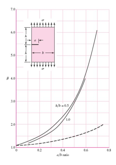
Beams of rectangular cross section having an edge crack.
